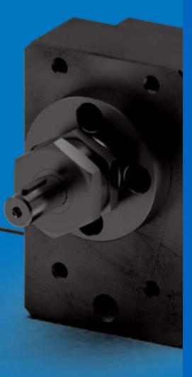
The PL2 can be considered a PL8 dressed for a party: thanks to the casing in heat-treated martensitic stainless steel is able to handle mildly corrosive fluids. It features a bigger shaft (16mm vs 12mm), a bigger support plate and centering dowels.
