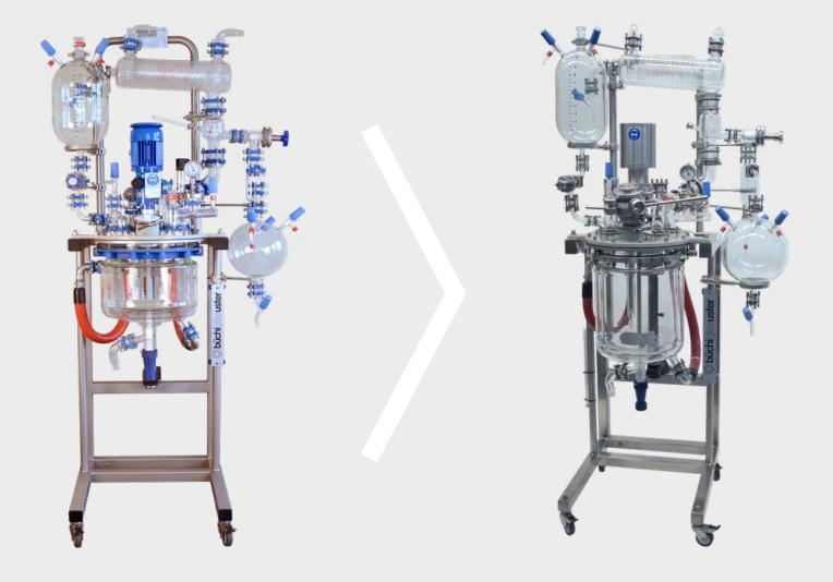
> Optimized cleanability of the relevant components due to polished surfaces in stainless steel
