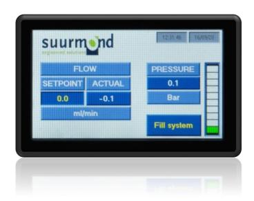
The control system has been developed as a universal solution to control fluid dosing in continuous processes.
