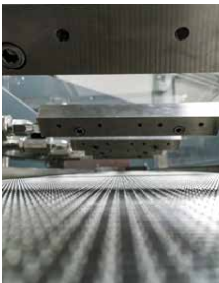
Air cooling nozzles
