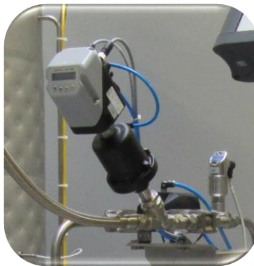
The pressure control valve simulates pressure using a PID control in the pump outlet.
