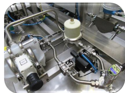
Membrane pump with pulsation damper to supply inlet pressure to the dosing pump.
