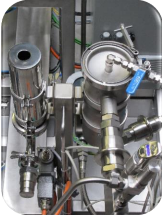
Filters can be exchanged without mess due to the Gather dry-break couplings.
