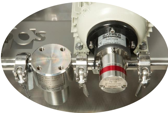
Gather dosing pump and HNP-M inline filter are mounted with tri-clamps
